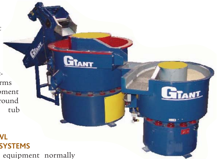
Figure 4: This photo shows two round-bowl vibratory systems being used in series. (An automated part feeder meters in parts.) After processing in an initial operation, parts can be separated and then transferred to either a secondary finishing operation or dried.
