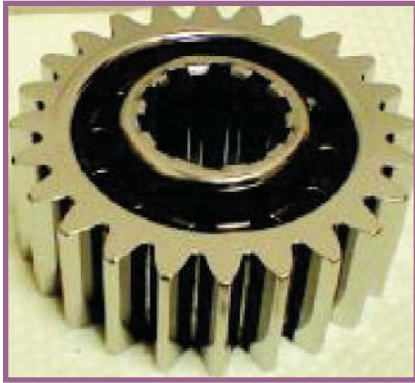
Figure 6: A number of companies utilize special chemistry to develop micro-surfaces to improve part performance in heavy load situations. These include conveyor chains, precision washers, forge dies, cast iron piston sleeves, camshafts, crankshafts, engine valves, and hydraulic pumps.
